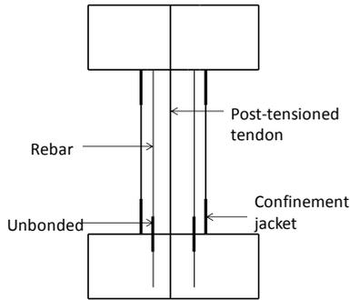
Figure 11. Post-tensioned hybrid rocking column
