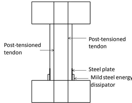
Figure 12. Hybrid rocking column with external ED bar
