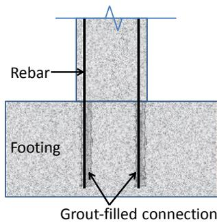
Figure 3. Grout-filled connection
