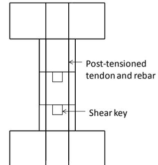
Figure 13. Hybrid rocking column with shear key
