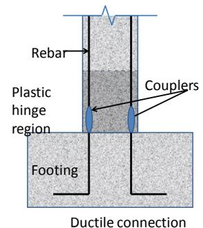
Figure 5a. Ductile coupler connection
