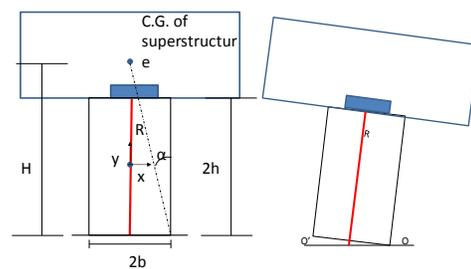
Figure 8. Restrained rocking column
