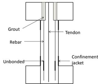
Figure 10. Pre-tensioned hybrid rocking column
