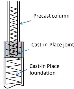
Figure 6. Deep foundation connection
