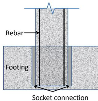
Figure 4. Socket connection
